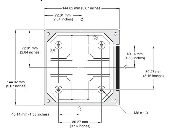
Figure 3-4 Panel Mount Cut-out Dimensions
